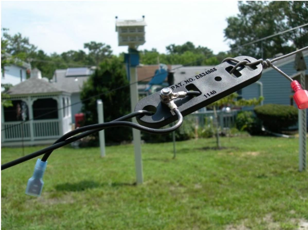
The grey AWG 16 wire is the 32 foot radial and a ¼ inch stab connector is crimped on the end. A stainless steel 5 mm stud is installed to terminate a jumper (with mating ¼ inch stab) and the 12 foot radial for 60 meters (black AWG 14). The other end of the black 12 foot radial is terminated in another insulator and is guyed to a ground stake.
